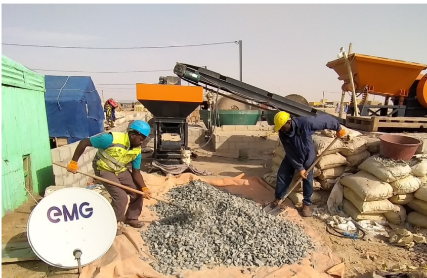
Picture 6: MAGMA team mixing the test ore batch, with shovels to ensure homogeneity
