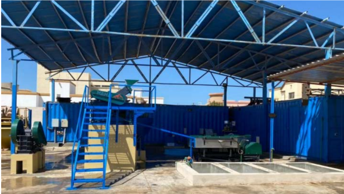
Figure 1. Magma’s mineral testing facility in Nouakchott where mineral processing equipment has been setup with support of the EPRM project for mineral test work, and for training ASM miners. Note that no mercury is used here and the facility is designed and used as a testing facility only (non-production). At right, note the engineered water recycling system, which has demonstrated a simple solution for water re-use.
