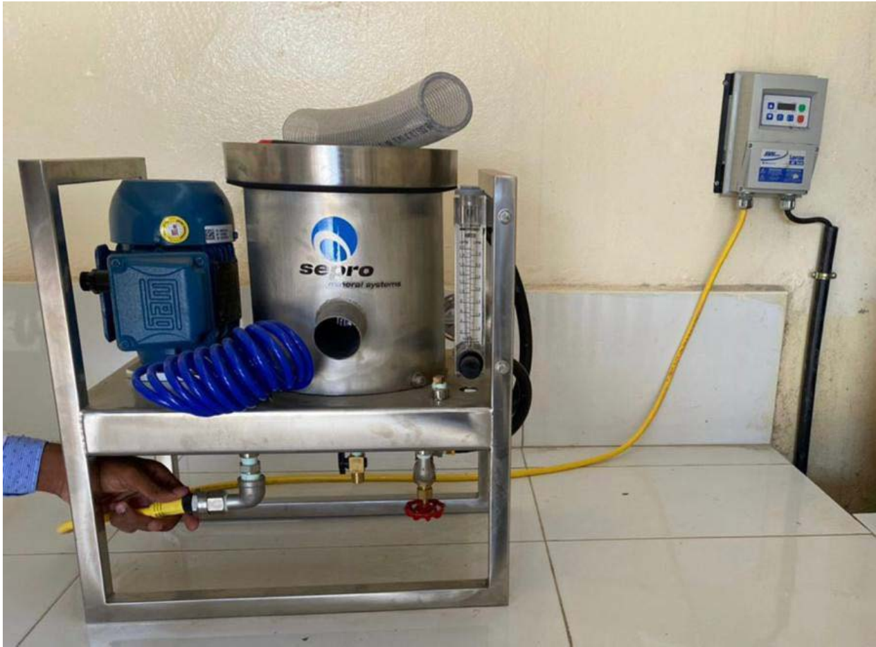
Figure 2. Sepro L40 laboratory-scale concentrator purchased from Falcon, in Canada.
