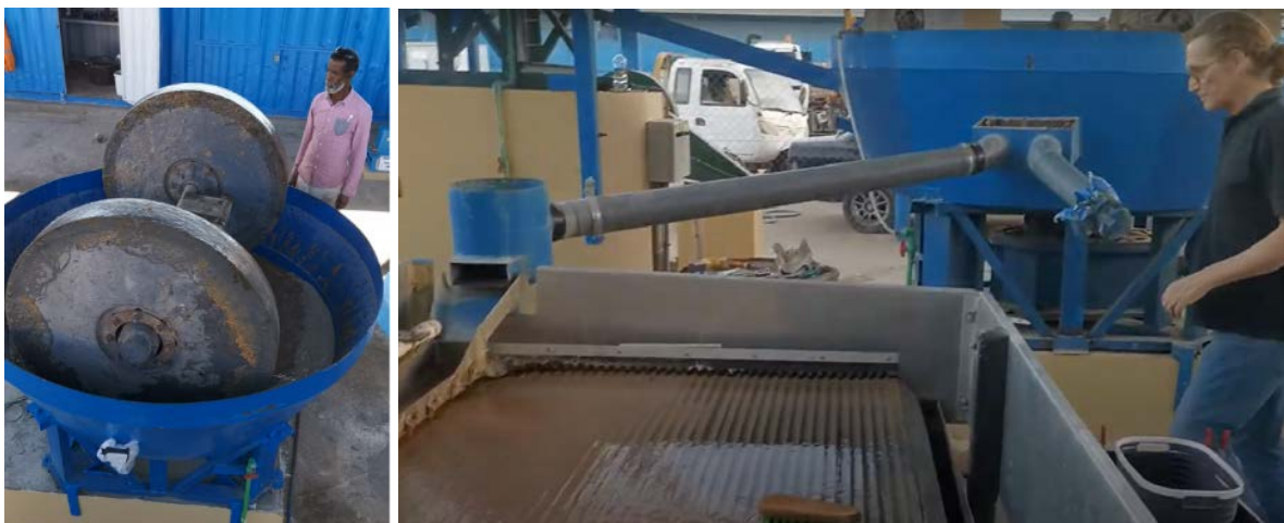
Figure 2. (left) The “wet-pan mill”, also known as “cone mill” (abbreviated WPM, herein) is the most widespread gold recovery technology used in Mauritania. (right) At the Magma yard, the WPM has been outfit with a custom port which allows slurry to run directly from the WPM to mineral concentrators: which can be: the shaking table (as shown above); or into the iCon150 (centrifuge); or directly onto sluice boxes (a method which is commonly employed in Mongolia).
