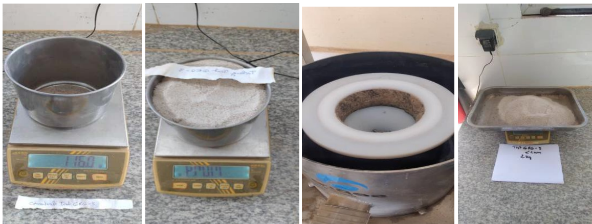
Figure 3. Various photos of milled ore samples : before, inside and after concentration with the L40 concentrator.
